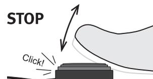
Press and hold the Foot Switch on and then turn the ON/OFF switch on. Lightly tap the foot switch to turn the e-Ball Winder ON and lightly tap again to turn it OFF. You can also operate your e-Ball Winder without the foot switch by turning it ON or OFF using the ON/OFF switch or speed control. However, our experience is that at full speed, the foot switch is a much more reliable way to stop tangles before they arrive at the yarn guide.
